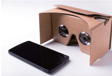
Google's Cardboard VR headset provides a VR experience with the LCD replaced by a smartphone. © misszin/Shutterstock
