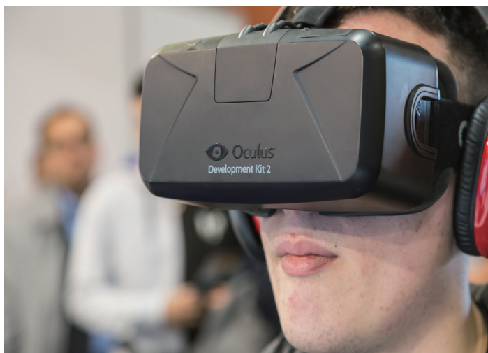
HMDs succeeded in realizing the human viewing angle of 120° but had yet to improve picture quality accordingly. © Tinxi/Shutterstock
