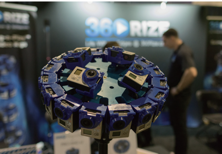
Images recorded from 360° are needed to realize VR. The above rig-type camera can record images in all directions. © betto rodrigues/Shutterstock
